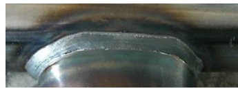
Mild steel / intersecting wire welding Thickness 1.5mm, Current 95A, Voltage 17V Welding speed 50cm/min Gas (20% Ar + 80% CO 2 )
